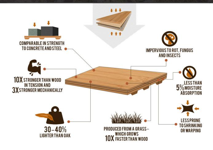
Prior to lamination, the veneers are dried and the grains of each veneer are oriented in the same direction. This makes LVB stronger, straighter and more uniform than solid timber and overcomes some of timber's natural limitation such as strength-reducing knots.
